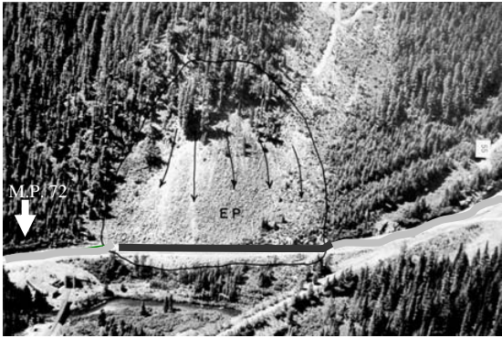
Figure 12: Slide guide shows aerial photos of all slide chutes. Area directly under slide path along the highway is colored red giving the operator a visual of where the danger area is in relation to the mile post marker.
