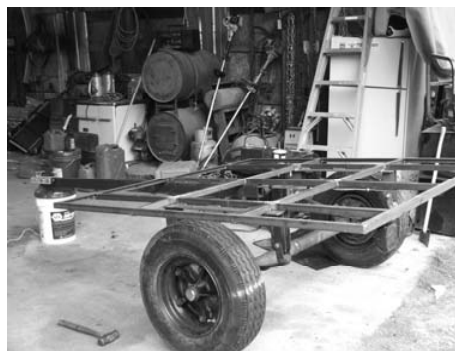
Figure 7: Axle and wheels were salvaged from the junk yard and bed was welded in one afternoon.
