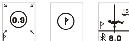
Figure 7: Left – The transmitter is pinpointed at 0.9 m depth. The user presses the MARK key. Center – The device acknowledges the MARK function. Right – The current transmitter is hidden, the next two buried persons in 8 m and 15 m distance, resp., are shown.
