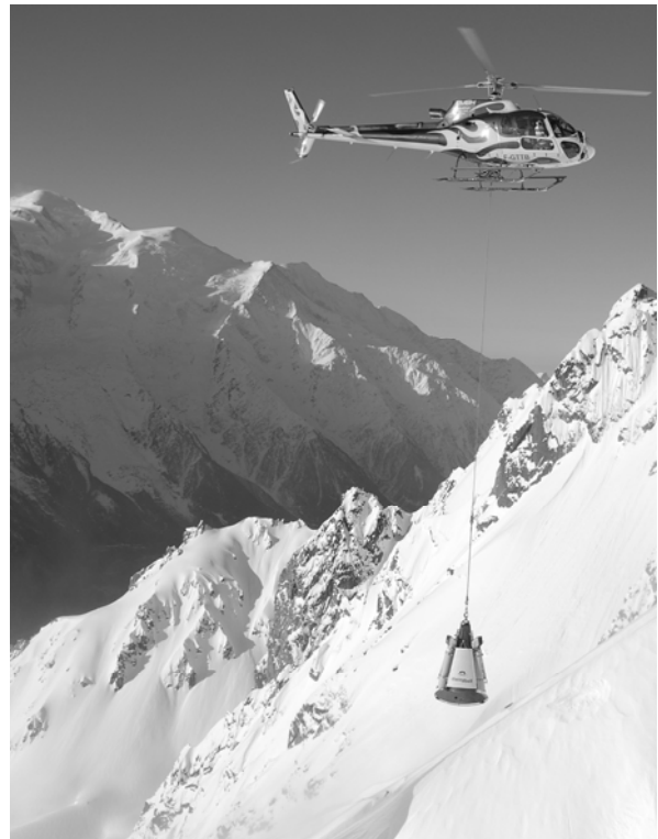
Figure 6: View of DaisyBell® in operation in the Chamonix Valley
