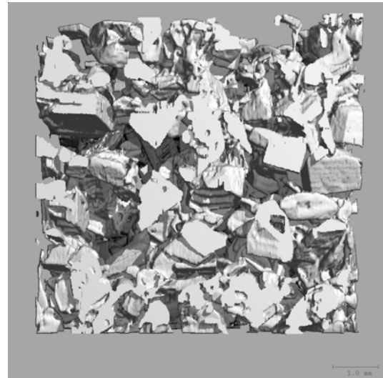
Figure 4: A three-dimensional reconstruction of snow formed through kinetic-growth metamorphism. Features such as hollow cups (hopper crystals) and scrolls are represented within the resolution of the model (voxel size is 12 \times 12 \times 12 \mu\text{m} ).
