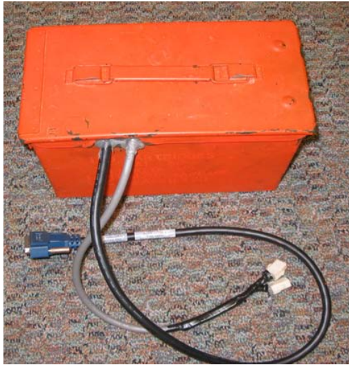
Figure 5. Surplus ammunition container enclosure containing data acquisition system.
