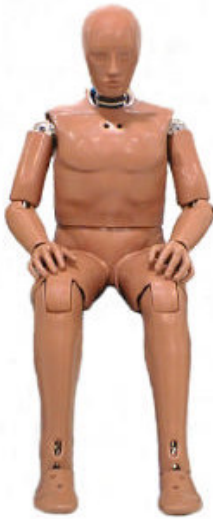
Figure 3. Hybrid III-50 th Percentile Crash Dummy standard configuration. Photo courtesy R.A. Denton, Inc.
