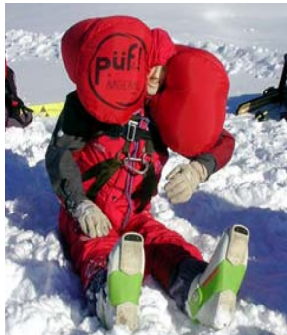
Figure 1: Dummies used in avalanche airbag testing at SLF, in 1994, 2001. Photos courtesy of the Swiss Federal Institute for Snow and Avalanche Research, Davos, Switzerland.
