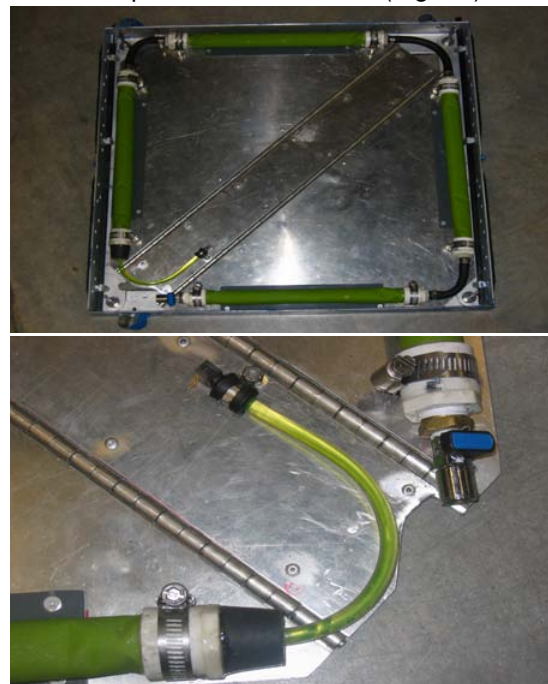
Figure 6. Portable fluid pressure load plate.
