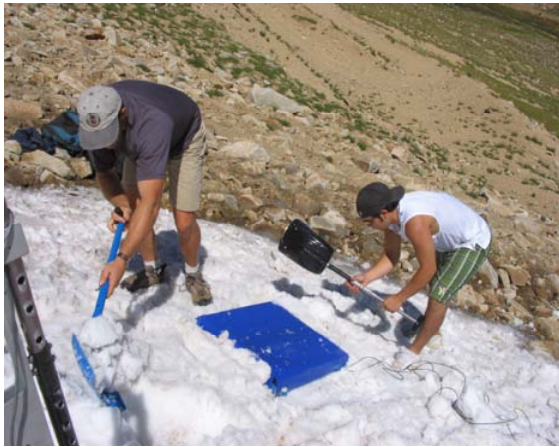
Figure 7. Portable fluid pressure load plate initial field testing. Photo by A. Yudell.
