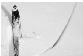
Figure 2: Photograph of a crack that suddenly shoots out from a ski. This indicates the presence of a slab and weak layer both of which are favourable to skier-triggered slab avalanches.
