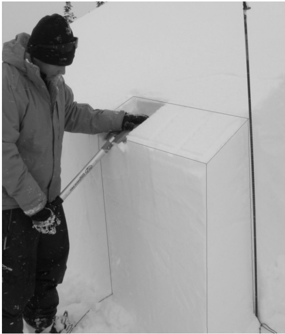
Fig. 2: Extended Column Test (ECT) in process. The operator is applying the same loading steps as for the standard compression test to one end of the column, noting when fractures initiate in a weak layer under the shovel and when they propagate across the column.
