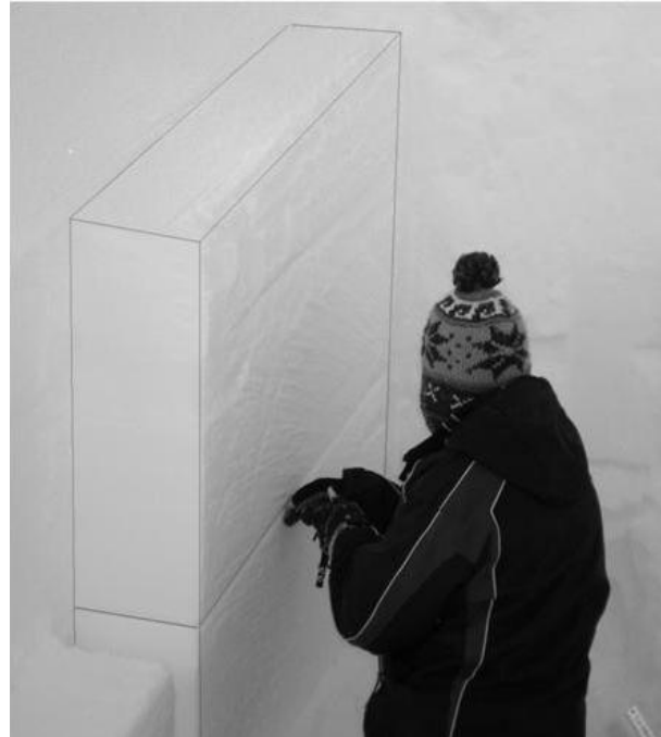
Fig. 1: Propagation Saw Test (PST) in process. The operator is drawing the blunt edge of a 2 mm thick saw upwards through the weak layer, stopping and marking the spot where the fracture propagates suddenly forward from the end of the saw cut.
