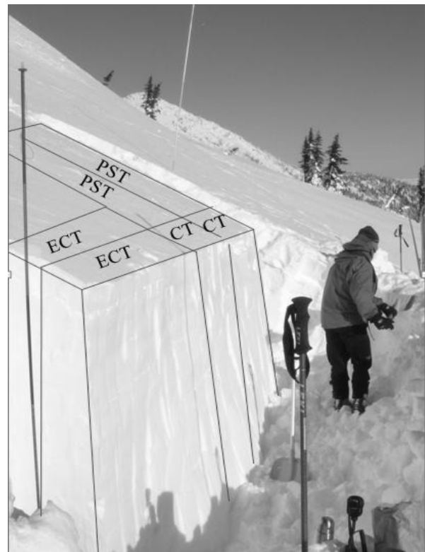
Fig. 3: Typical pit layout for comparing the PST and ECT
