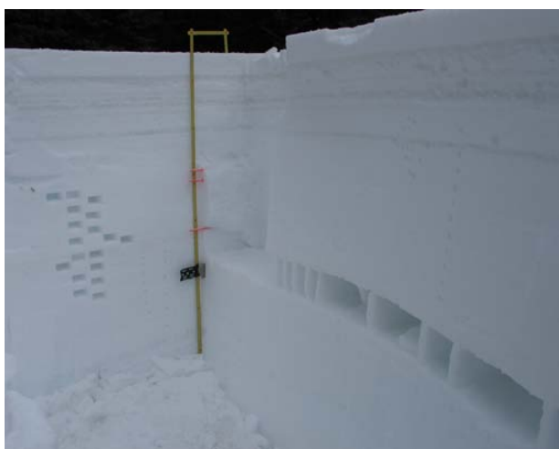
Figure 1: Photograph of a snow pit after a standard profile observation and extraction of samples. Samples of different sizes were taken from a slab layer that extends from the lower right corner of the picture.
