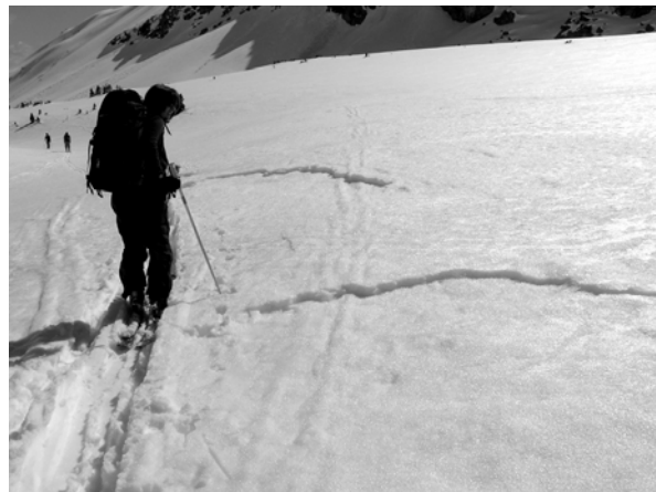
Figure 2. A researcher investigates the perimeter slab fracture surrounding a small whumpf. Note the radial propagation pattern from the trigger point (foreground), which is distinct from the more two-dimensional geometry of the PST (e.g. Figure 1). (Bruce Jamieson photo)
