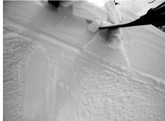
Figure 1. Example of the excavation of a test-skiers tracks where no avalanche resulted. In this case, weak layer damage below the skis indicates that a fracture was initiated, but did not propagate. (ASARC photo)
