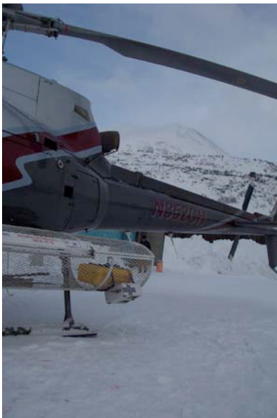
Figure 1. Helicopter-mounted FMCW radar measurements. 2-10 GHz radar is white box on outside of ski basket, yellow case contains rugged tablet computer.
